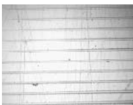
Parallel scratches on gold film on glass with 5 \mu\text{m} spherical indenter with loads 5, 10, 15, 20... mN at 5 \mu\text{m} intervals.
