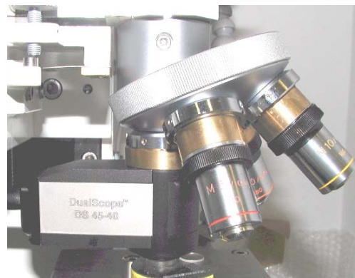
AFM Objective fitted to optical microscope
